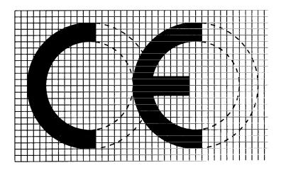
If the marking is reduced or enlarged, the proportions given in the above graduated drawing must be respected.
